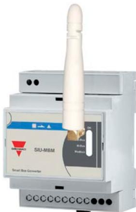
The gateway/receiver offered by Carlo Gavazzi is SIU-MBM-02, which is able to integrate up to 20 wired devices and 32 wireless devices and can transmit data via Modbus TCP/IP (Ethernet port).
